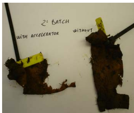
Figure 6: Samples from batch 2 (using accelerator) and batch 3 (without using accelerator) after 1.5 months
